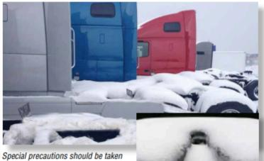
during extreme cold weather to ensure that the fifth wheel locking mechanism operates freely. At low temperatures ice and sludge can build up, and lubricants can become
